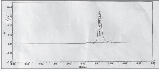
Figure 2 Typical Chromatogram (Pure DOX, 300 µg/mL).
